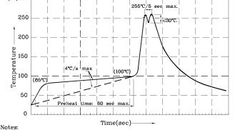
I.Recommend pre-heat temperature of 105°C or less (as measured with a thermocouple attached to the LED pins) prior to immersion in the solder wave with a maximum solder bath temperature of 260°C
